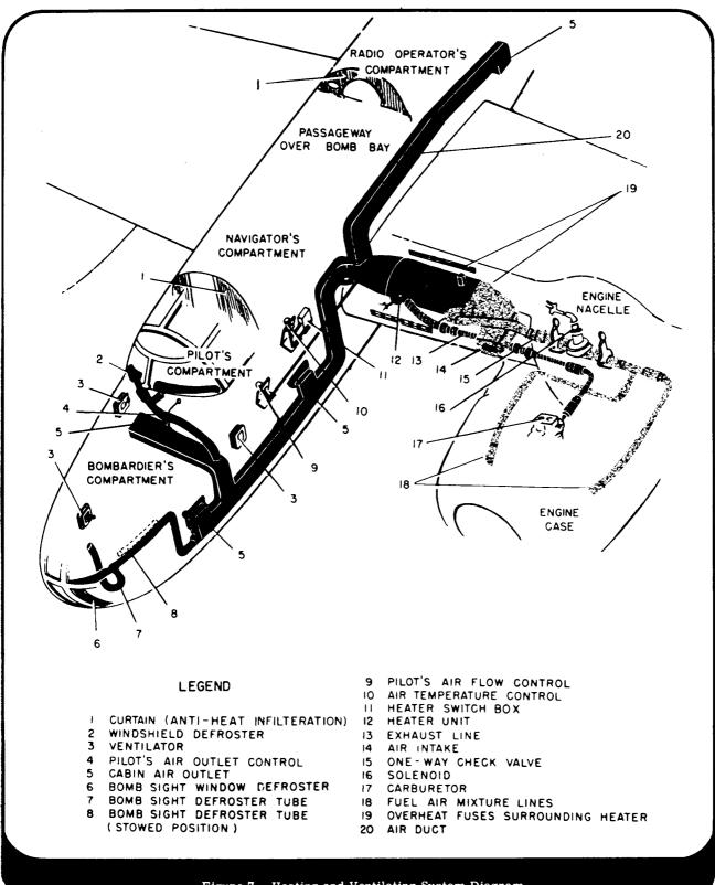
Figure 7 - Heating and Ventilating System Diagram
