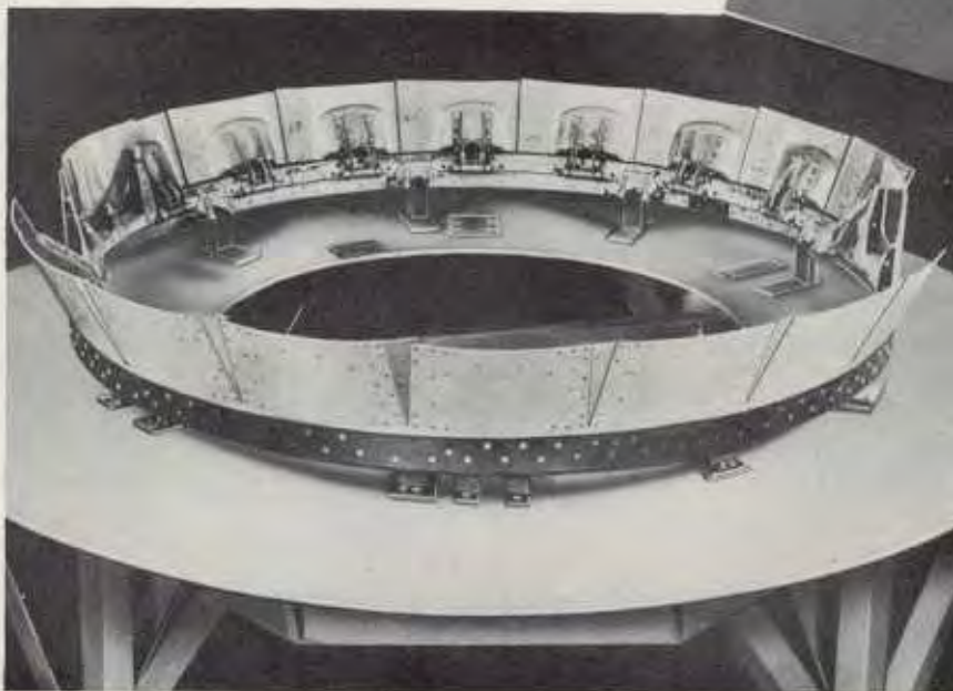
Figure 92—Engine Cowl Ring Flap Construction (15-7655)
