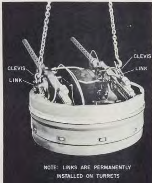
Figure 284—Hoisting Upper Turret
