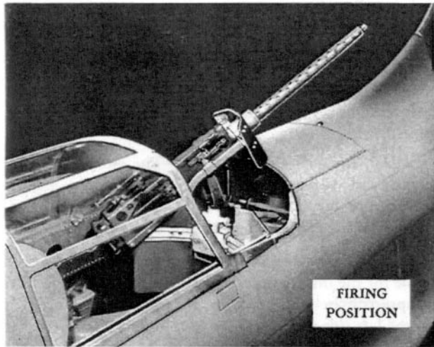
Figure 41—Upper Flexible Gun in Firing and Stowed Positions
